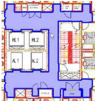
Polyline being recognized in iTWO costX®
